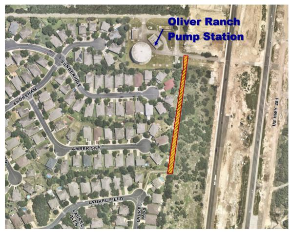
The project includes approximately 677 LF of 16-inch DI main to be installed within an existing variable width water easement and will tap an existing 24-inch water main.
